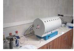
EN 50267-2-3:1999 / BS EN 50267-2-3:1999 / DIN EN 50267-2-3:1999 / VDE 0482-267-2-3:1999-04 / CEI EN 50267-2-3:1999 (CEI 20-37/2-3). Common test methods for cables under fire conditions-Test on gases evolved during combustion of materials from cables- Part 2-3:Procedures. Determination of degree of acidity of gases for cables by determination of the weighted average of pH and conductivity.
