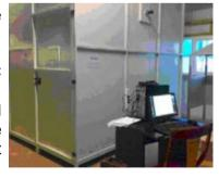
IEC 61034-2:2005 / EN 61034-2:2005 / BS EN 61034-2:2005 / DIN EN 61034-2:2006 / VDE 0482-1034-2:2006 / CEI EN 61034-2:2006 (CEI 20-37/3-1) Measurement of smoke density of cables burning under defined conditions.
